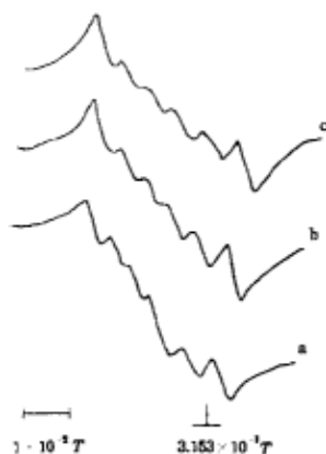
图 2 Mn-SIIR 溶液在不同浓度时的 ESR 谱 Fig.2 ESR spectra for Mn-SIIR in xylene with 5% hexanol at concentration of (a) 0.5, (b) 1.0 and (c) 2.0g·dL -1
