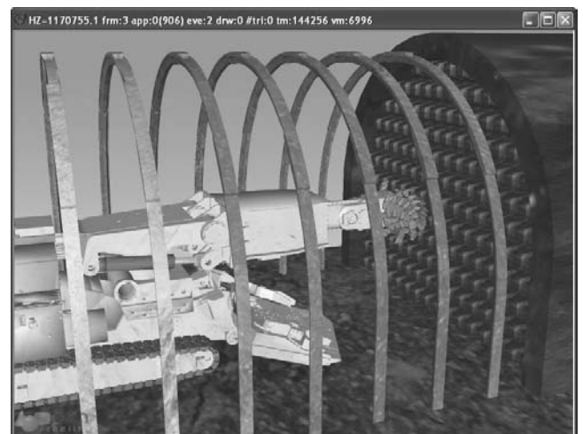
Fig. 5. 3D model of roadheader
