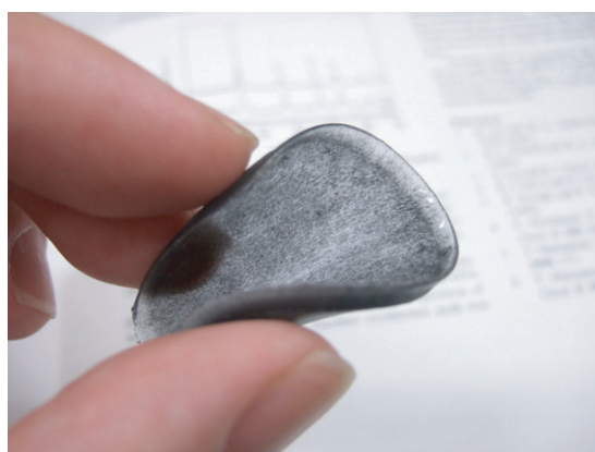
Figure 7. Horizontal alignment of CNTs in silicone composite.
