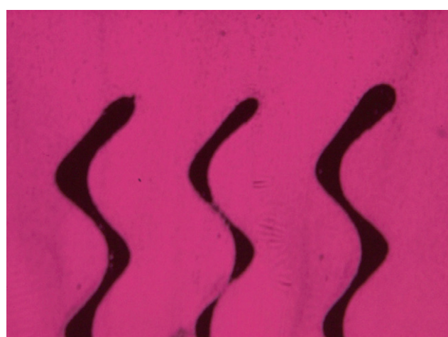
Figure 14. The three wave lines indicate that CNTs are aligned perpendicular to each other.
