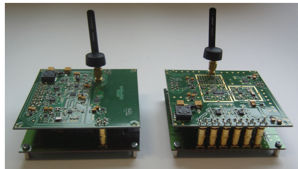
FIGURE 8: MARS receive and transmit boards.
