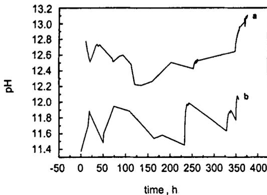
Fig. 6 Time dependence of pH at the steel/concrete interface in 3% NaCl. IrO<sub>2</sub> - pH sensor was installed at the interface (a) before the cement paste was hardened, and (b) for the hardened paste
