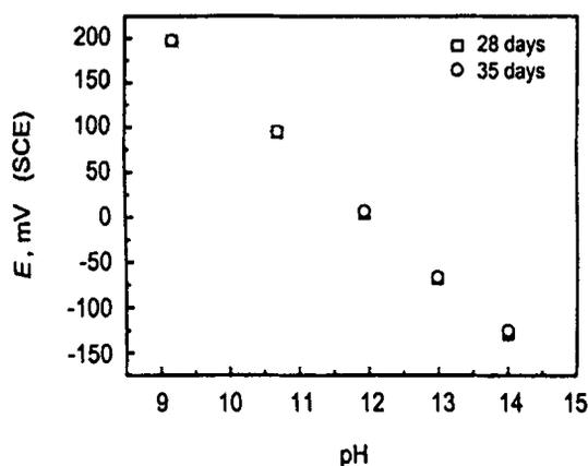
Fig. 4 Potential - pH diagram for an aged Ir/  $\text{IrO}_2$  electrode treated by carbonate (aged for 28 and 35 days)
