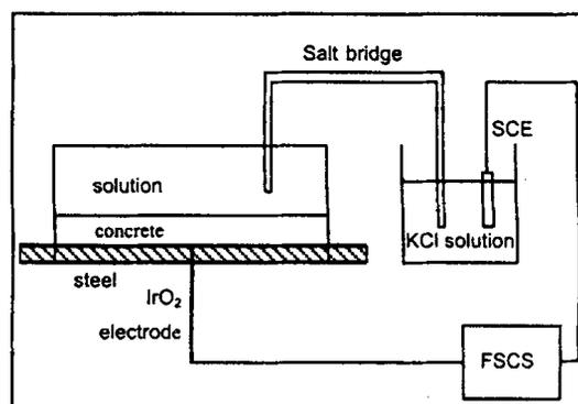
Fig. 1 Arrangement for measuring pH at the interface of reinforced steel/ concrete by IrO<sub>2</sub> electrode
