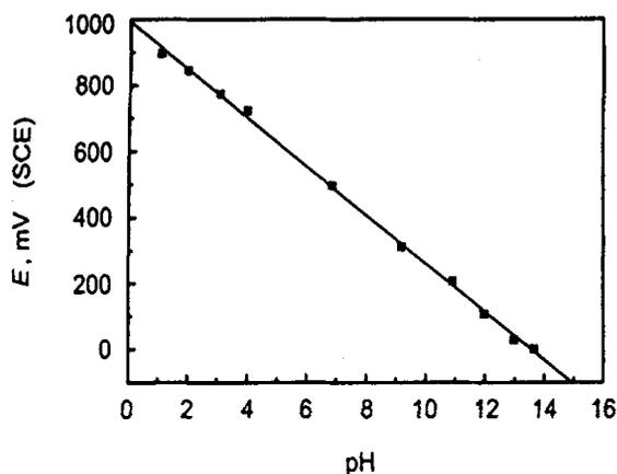
Fig. 3 Potential - pH diagram for a fresh Ir/  $\text{IrO}_2$  electrode treated by carbonate at high temperature
