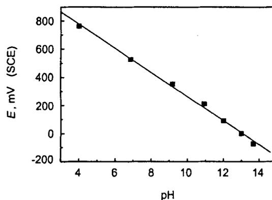
Fig. 2 Potential - pH diagram for a fresh Pt/ IrO<sub>2</sub> electrode prepared by anodic electrodeposition
