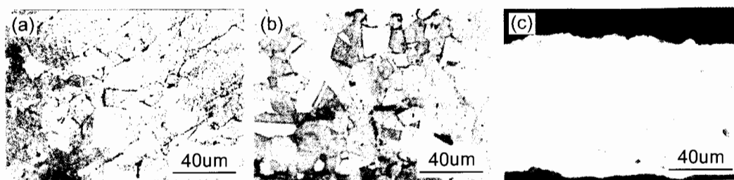
Fig. 2 Optical micrograph of failed components. (a) baffle plate of the third crystallizer; (b) baffle plate of stripper-distillation column; (c) component of solvent stripper
