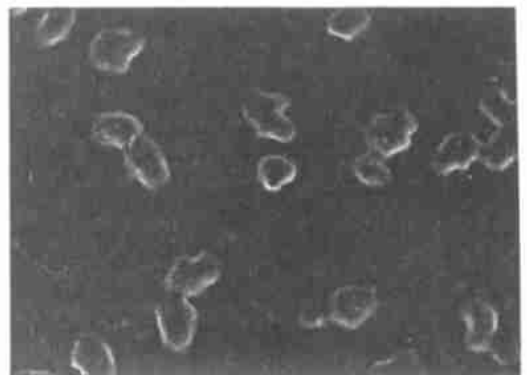
Fig. 1 SEM photo of alkyd coating after 14d exposure under RH 100%, x100
