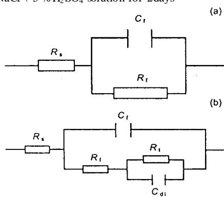
**Fig. 6** Equivalent circuits of coated electrode
