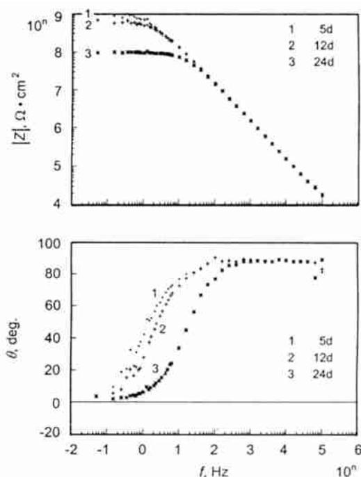
Fig. 3 Bode diagram of no. 2 electrode after immersion in 3.5 % NaCl solution for different times
