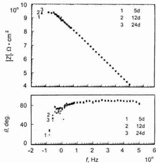
Fig. 4 Bode diagram of no. 3 electrode after immersion in 3.5 % NaCl solution for different times
