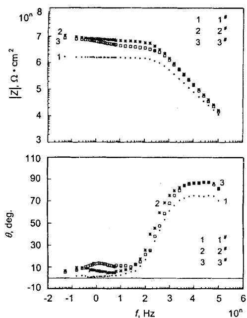
**Fig. 5** Bode diagram of different electrodes after immersion in 3.5% NaCl solution for 24 days, then immersion in 3.5% NaCl + 5% H<sub>2</sub>SO<sub>4</sub> solution for 2 days
