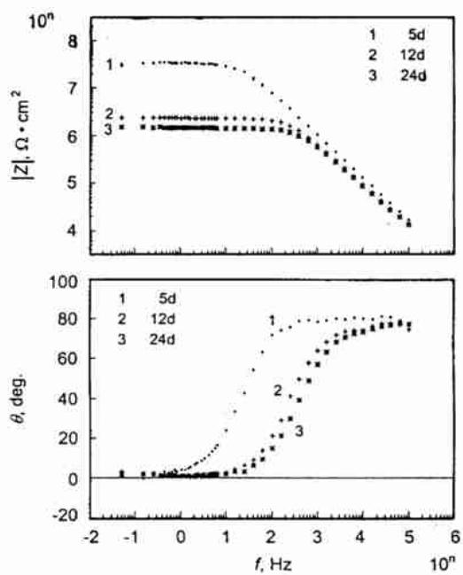
Fig. 2 Bode diagram of no. 1 electrode after immersion in 3.5 % NaCl solution for different times
