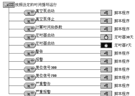
图5 油气回收装置监控软件循环策略窗口 Fig.5 Oil and gas recovery cycle monitoring software strategy window
