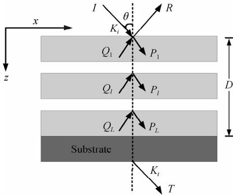
Fig. 1 Geometry for the reflection and transmission of multi-layer optical dielectric thin film
