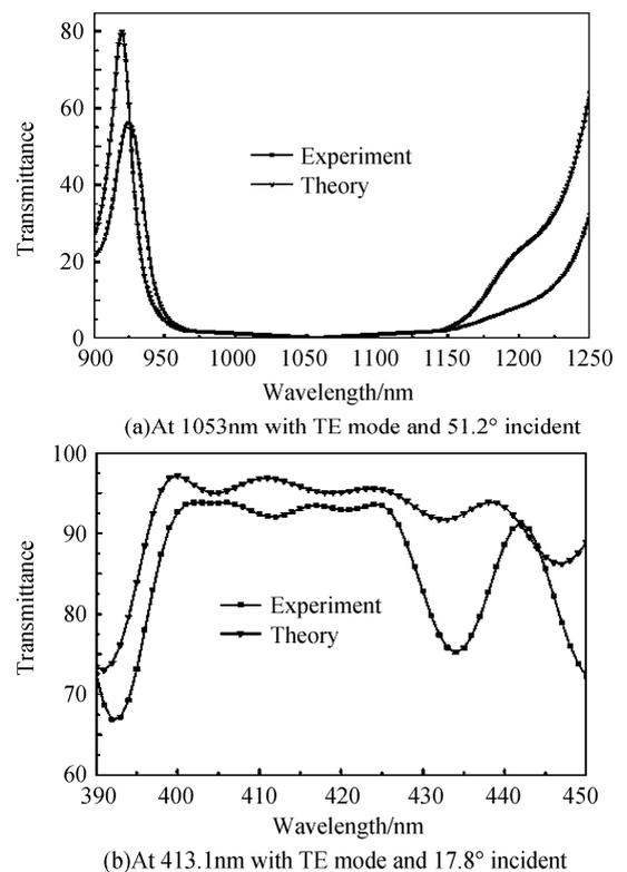
Fig. 2 Optical performance of  $H_3L(H_2L)^9H_0.5L$
