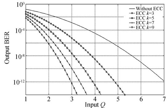
Fig. 3 Input Q vs output BER
