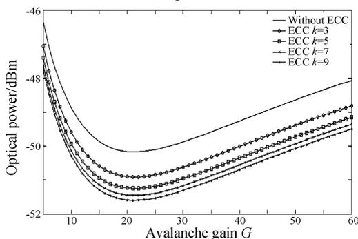
Fig. 5 Receiver sensitivity of PWAM system with ECC
