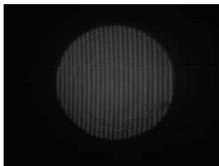
图3 相机焦平面处干涉图 Fig. 3 Interferogram on the focal plane of camera
