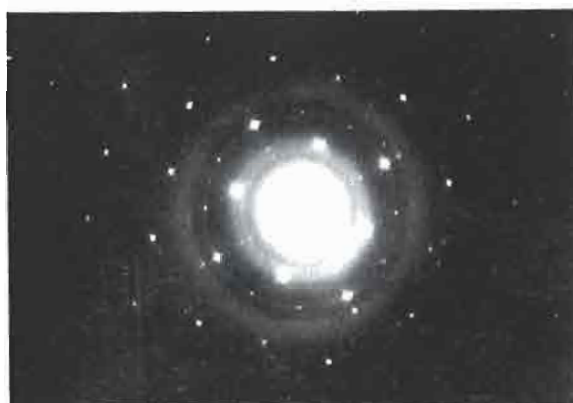
Spot diffraction pattern from orientated crystals after heat treatment of the initial film for 1 hour at 450°C in air
