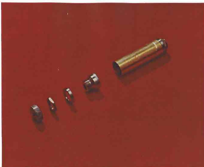
Fig. 2 Exploded view of a typical capsule assembly. Gold tubing has the ability to deform under high pressure without rupturing. Gold is also fabricated easily into the capsule, it is inert to most reactants, and its high melting point permits it to withstand exothermic reactions of the reactants
