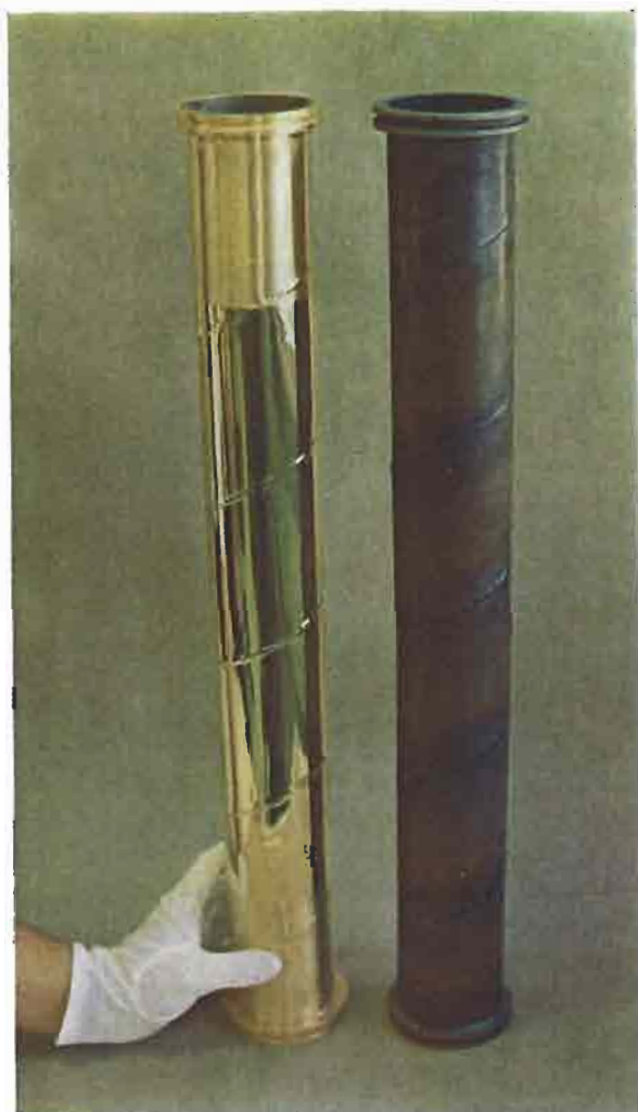
Tubes coated with gold and with p-xylylene polymer for tests in a vertical tube still at the Wrightsville Beach Test Facility of the Office of Saline Water
