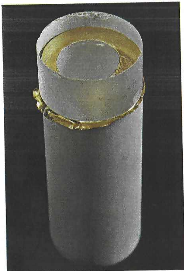
Fig. 3 A close-up view of the bond in the spectrographic cell made from an alumina container with sapphire windows
