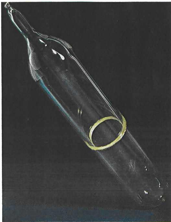
Fig. 4 An example of a vacuum-tight seal made by reaction welding. This Pyrex/gold/Pyrex test assembly has been maintained for eighteen months under a vacuum of 10^{-6} torr
