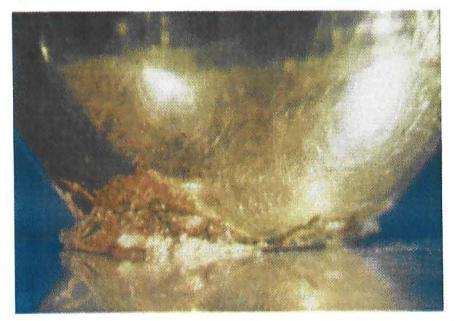
If the flat surface is much harder than the gold, as is the case with rhodium, a small amount of the gold may transfer back and forth between rider and flat with no prow formation and little wear resulting. (Direction of movement from left to right)
