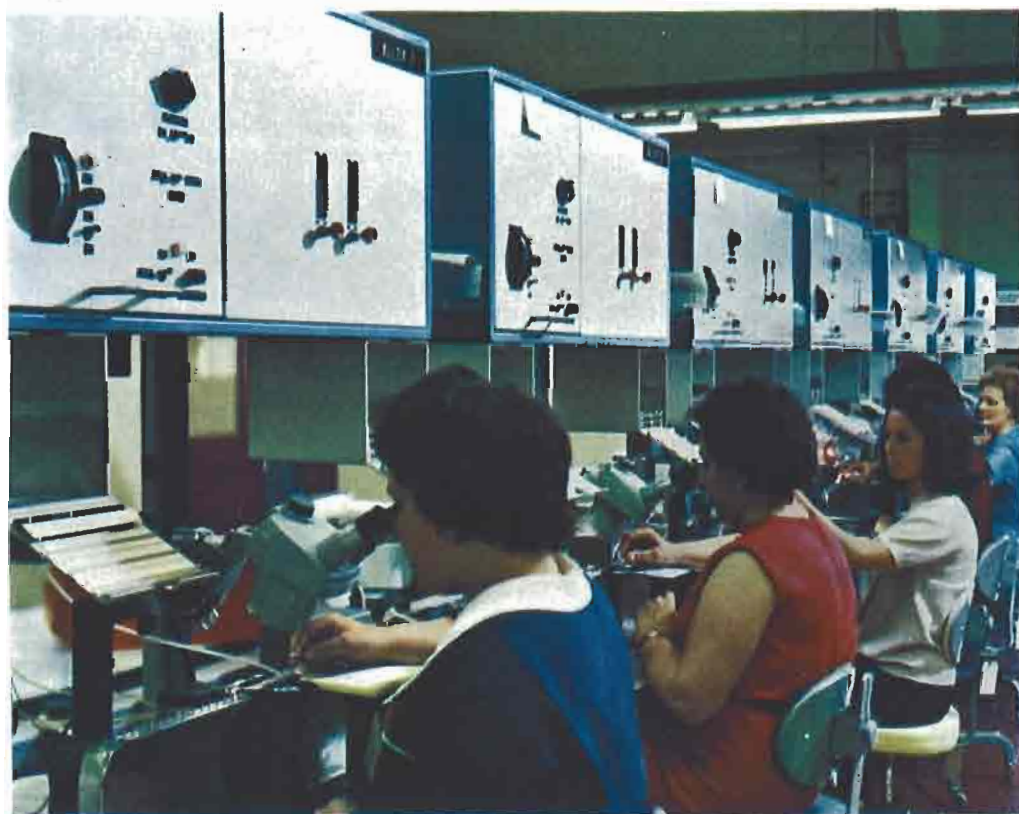
The bonding stage in the production of integrated circuits at Texas Instruments. Gold lead wires are being connected to the metallised area of the silica slices.
