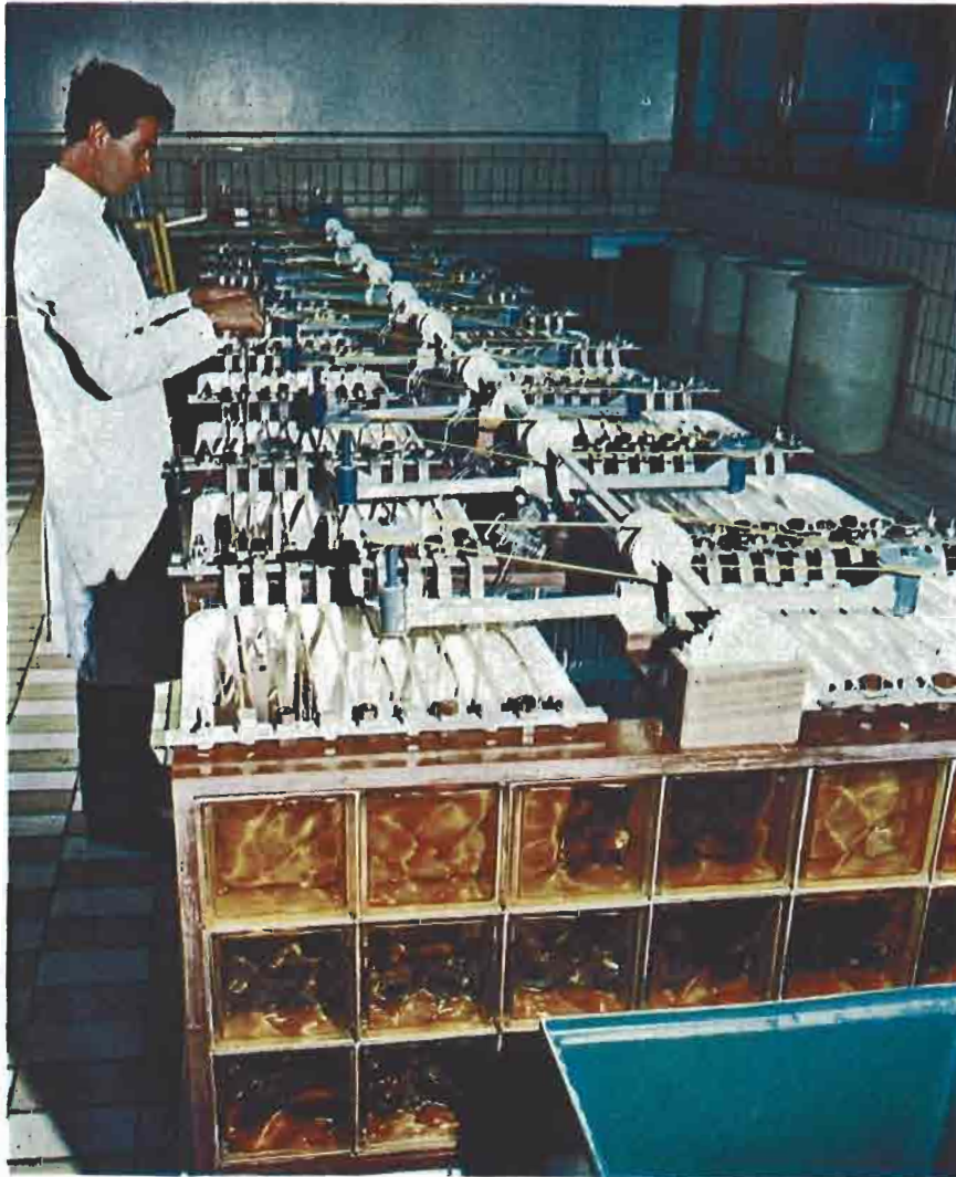
A small electrolytic refinery has been installed in the new plant to produce gold of 99.99 per cent purity for specialised industrial uses.
