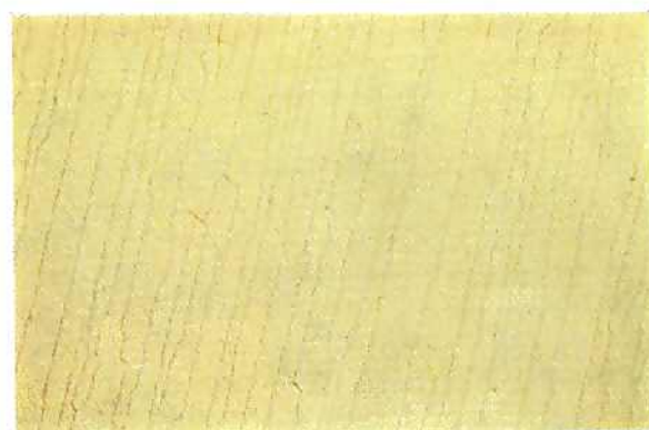
Fig. 2 Alloy ACZ2 (57% Au, 15% Cu, 28% Zn) in the cast state. Each grain contains many narrow sub-grains; the fine martensitic structure can be seen within each sub-grain ×100
