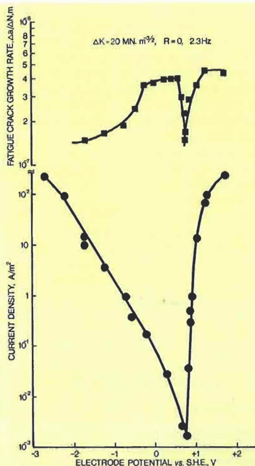
Fig. 4 The application of an electrical potential (expressed here vs. a standard hydrogen electrode) has a marked effect on the growth rate of fatigue cracks in a specimen of 95 gold/5 nickel weight per cent alloy exposed to a 5 molar aqueous solution of sodium chloride (pH 6) at 23^\circ\text{C} . The sharp minimum recorded in the fatigue crack growth rate at +750 \text{ mV vs. SHE} is reproducible but still has to be explained
