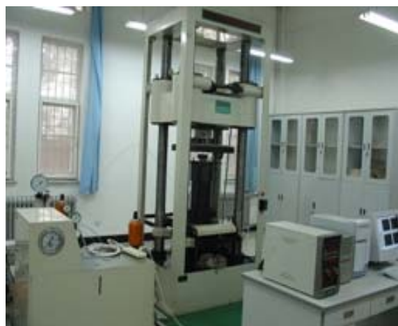
图 1 XTR01-01 型微机控制电液伺服岩石三轴试验仪 Fig.1 Microcomputer electro-hydraulic servo-controlled triaxial test machine XTR01-01
