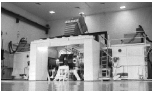
Fig. 3 High-repetition-rate electron-beam-pumped KrF laser "Electra" at NRL.
