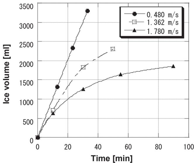
Fig. 3. The effect of circulation flow rate on growth rate of ice formation of pure water in a tubular ice system (coolant temperature =  $-5^\circ\text{C}$ ).
