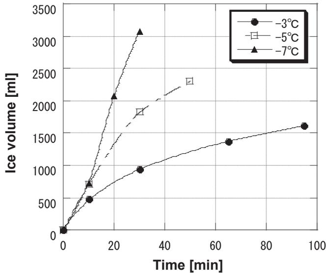
Fig. 2. The effect of coolant temperature on growth rate of ice from pure water in a tubular ice system ( $v = 1.362 \text{ m/s}$ ).
