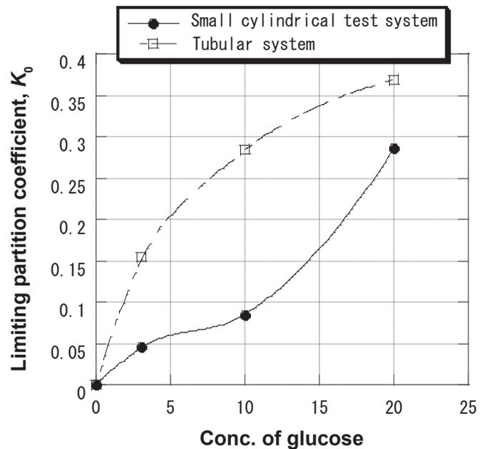
Fig. 5. The effect of solute concentration on limiting partition coefficient for a tubular system and a small cylindrical test system for progressive freeze-concentration.
