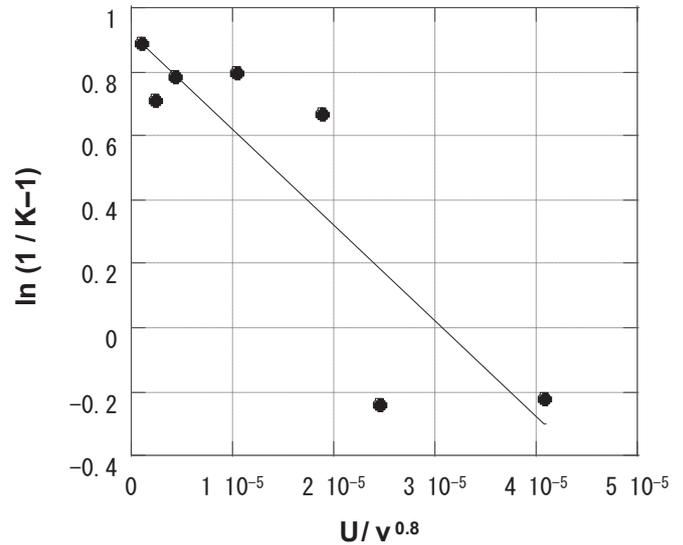
Fig. 4. Plot for limiting the partition coefficient for 10% glucose solution in a tubular system for progressive freeze-concentration.
