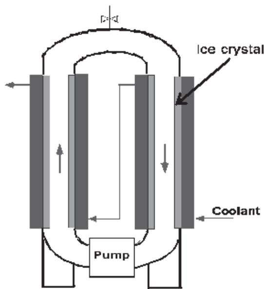
Fig. 1. A tubular ice system for progressive freeze-concentration.
