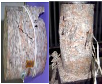
图 7 反复加卸载后破坏的单轴压缩试件 Fig.7 Failure samples after cyclic loading and unloading under uniaxial compression
