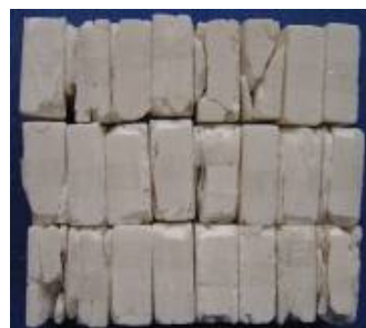
图 14 双向压缩破坏后大理石试件 Fig.14 Marble samples after bi-compression failure
