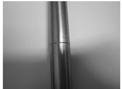
图9 含环向裂纹缺的传热管 Fig. 9 SG tube with circumference crack defect
