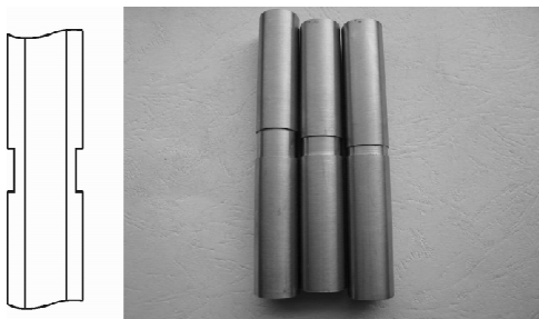
图6 含环向1圈缺陷的传热管 Fig. 6 SG tube with whole loop defect
