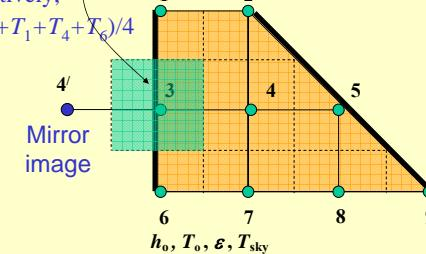
**Solution:** Energy Balance:  $\sum_{\text{all side}} \dot{Q} + \dot{g}V_{\text{element}} = 0$
