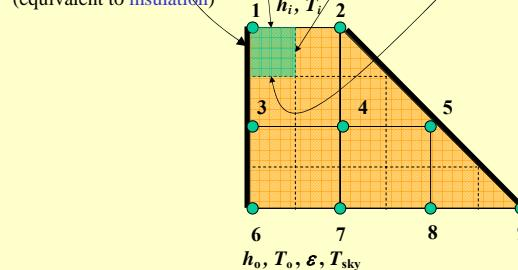
**Solution:** Energy Balance:  $\sum_{\text{all side}} \dot{Q} + \dot{g}V_{\text{element}} = 0$
