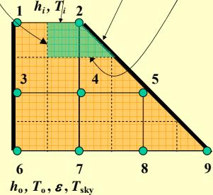
**Solution:** Energy Balance:  $\sum_{\text{all side}} \dot{Q} + \dot{g}V_{\text{element}} = 0$
