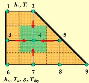
**Solution:** Energy Balance:  $\sum_{\text{all side}} \dot{Q} + \dot{g}V_{\text{element}} = 0$
