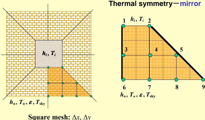
Solution: Energy Balance:  $\sum_{\text{all side}} \dot{Q} + \dot{g}V_{\text{element}} = 0$
