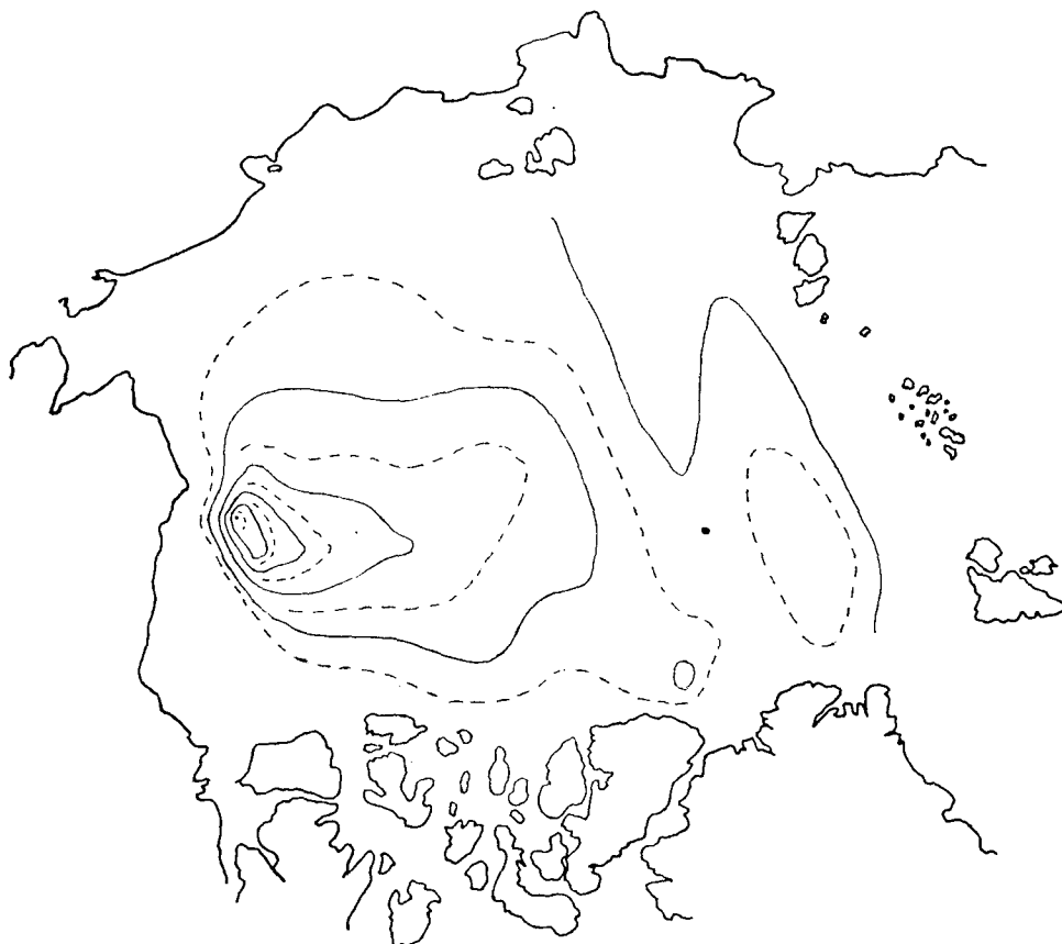
FIG. 11. Streamline pattern for the wind-driven case after 600 days. Non-linear terms, bottom and lateral friction, inflow-outflow on the boundaries, and 10% of the bathymetric variation are included. Between solid lines the transport is 10^7 \text{ m}^2 \text{ sec}^{-1} .
