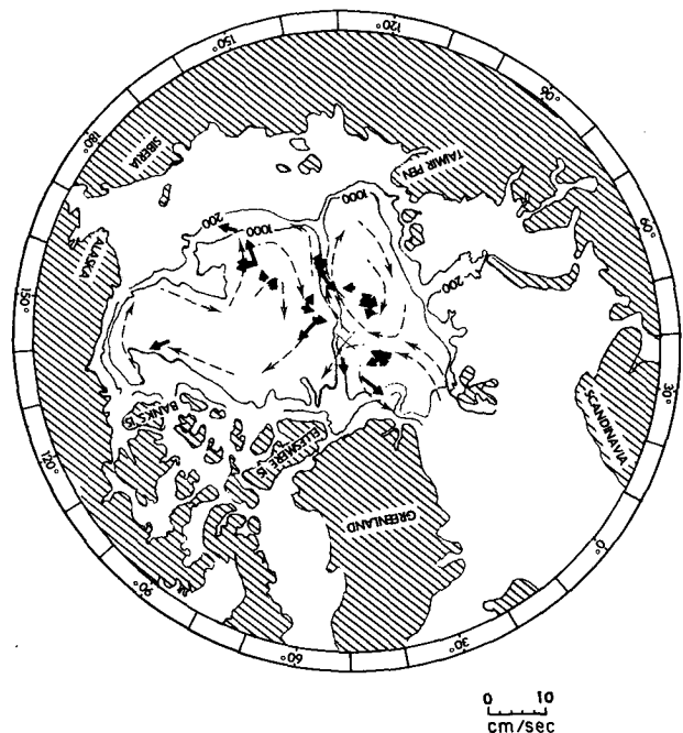
FIG. 10. Schematic view of Atlantic layer circulation (dashed arrows) predicted by Case III of the model, with direct current measurements (solid arrows) compiled by Coachman and Aagaard (1974). The velocity scale at the lower right is for the observed currents.
