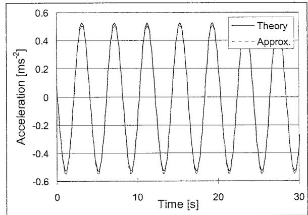
Fig.A1 Time histories of lateral acceleration obtained from theoretical and approximate equations.
