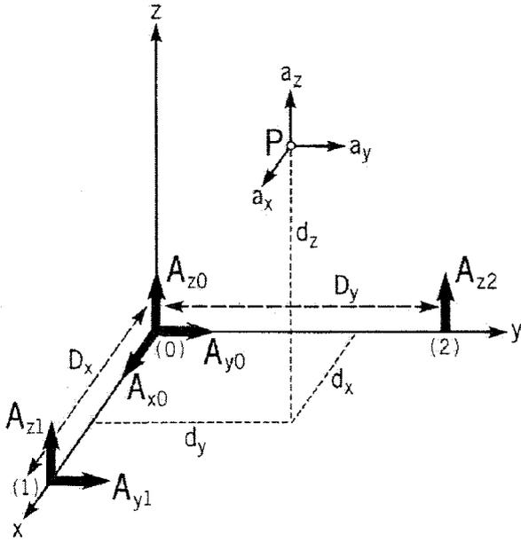
Fig.3 Accelerometer locations and orientations for calculating the six axes of motion at arbitrary point P<sup>6)</sup>.
