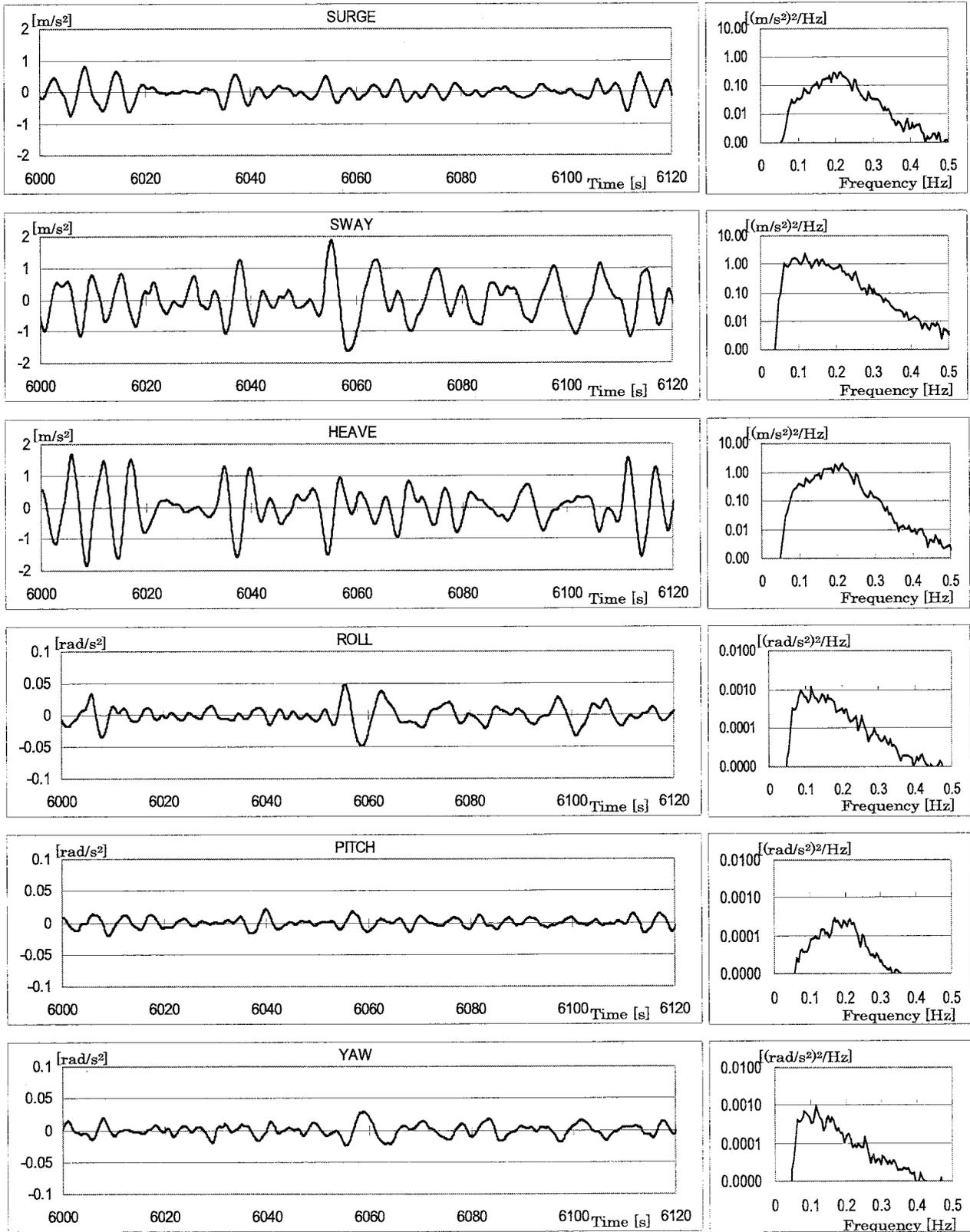
Fig.4 Acceleration time histories (a) and power spectral densities (b) for the six axes of motion of the 'Vena': frequency resolution 0.0049 Hz; duration 1500 seconds.
