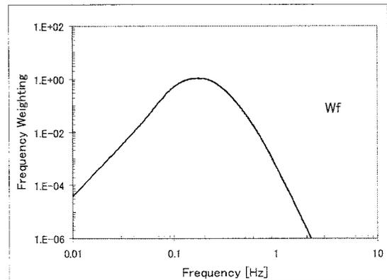
Fig.5 Frequency-weighting curve  $W_f$  defined in ISO 2631-1.
