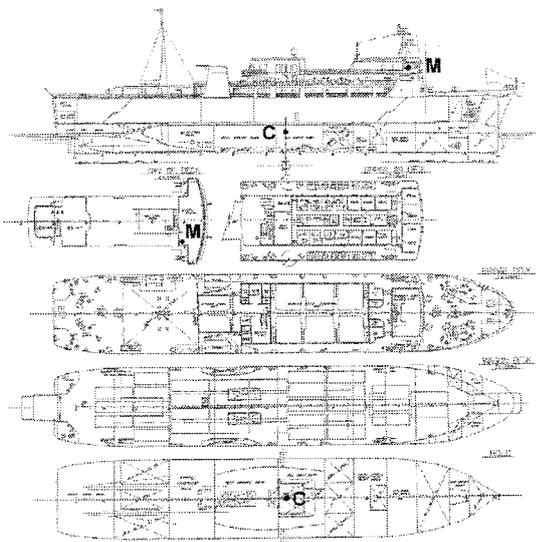
Fig.1 General arrangement of the 'Vena'. Ship motion was measured at the point M in the navigation bridge, and 6-degrees-of-freedom of motion at the point C was calculated for evaluating ride comfort.
