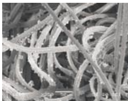
Figure 4. Image of the viscose nonwoven with microspheres incorporated by the spraying method, obtained with the use of a Jeol JSM5500C scanning electron microscope.
