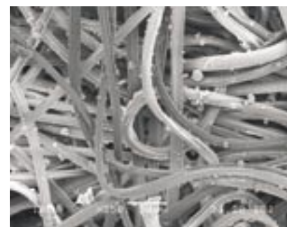
Figure 5. Image of the viscose nonwoven with microspheres incorporated by the pouring method, obtained with the use of a Jeol JSM5500C scanning electron microscope.
