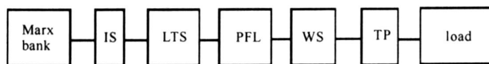
IS; intermediate store; LTS; laser triggered gas switch; PFL; pulse forming line; WS; self-breaking water switch; TP; water insulated tri-plate transmission line
