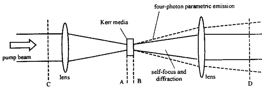
Fig. 4 Schematic of experimental setup
