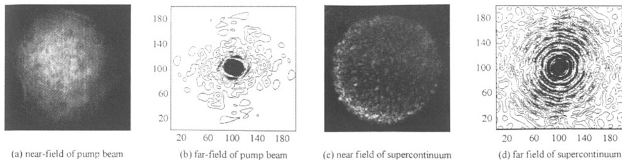
Fig. 5 Near-field and far-field patterns of pump beam and supercontinuum
