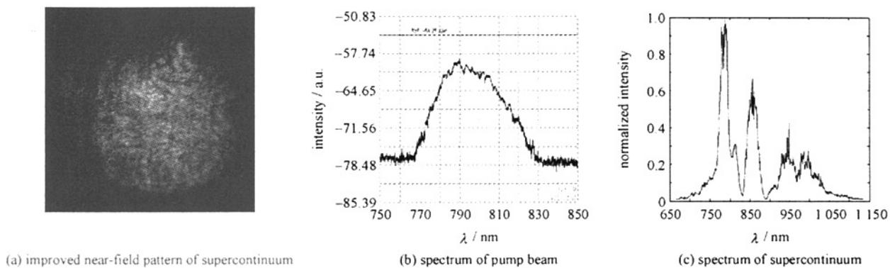
Fig. 6 Spectral distribution of pump beam and supercontinuum
