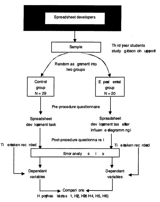
Figure 4. Schematic representation of the experimental method
