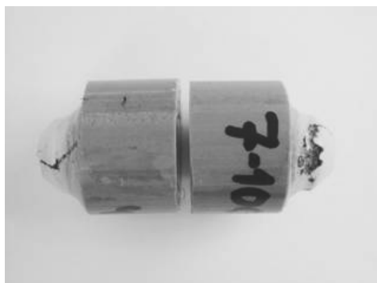
Fig. 3. Microscope view of samples with barriers type TBC, after having been tested by cyclic oxidation and preliminarily mounted in cold
