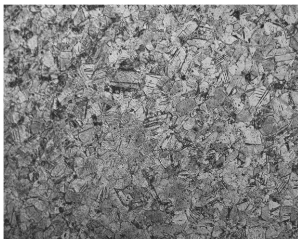
Fig. 2. Structure of the investigated steel after deformation with a draft of 17%; Etching - Mi17Fe; Mag. 200x
