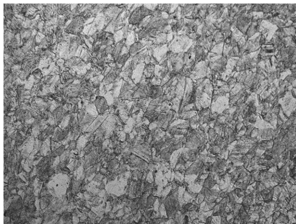
Fig. 3. Structure of the investigated steel after deformation with a draft of 33%; Etching - Mi17Fe; Mag. 200x
