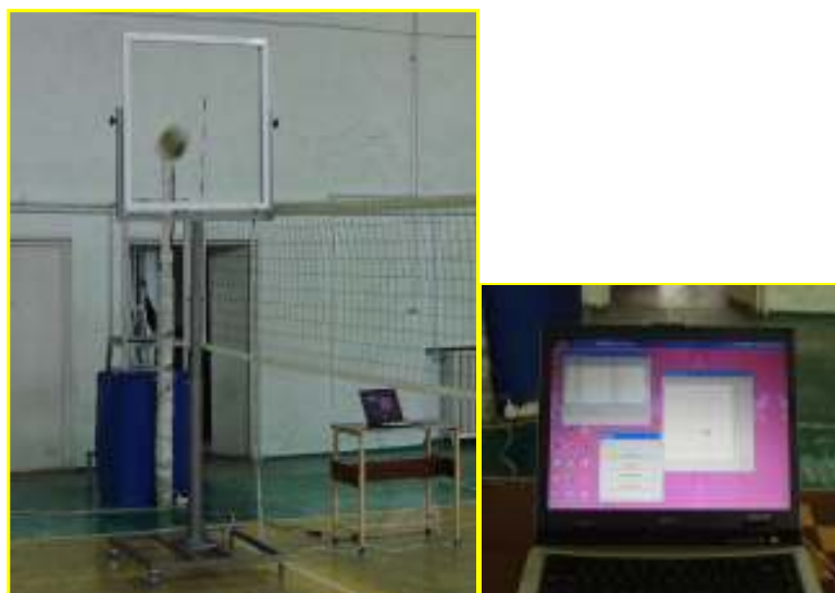
Figure 1. The DIRPAS-NS2006 system - the mechanical support, the testing framework, the local electronic block, PC and the interface with the user.
