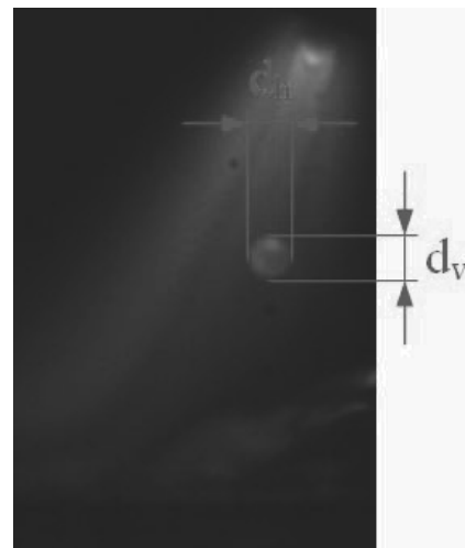
Fig. 6. Methodology for calculating the diameter of a single droplet in GMAW. d_h – horizontal diameter, d_v – vertical diameter
