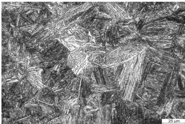
Fig. 4. Bainitic-ferritic microstructure of the 0.24%C steel containing retained austenite cooled with a rate of 7^{\circ}\text{C}\text{s}^{-1} from 900^{\circ}\text{C}
