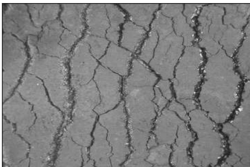
Fig. 4. A grid of cracks on the surface of of hot rolled alloy at a temperature of 1200-1100°C at alloy without spacers
