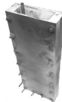
Fig. 6. Mould for plain specimen a) graphite inner mould, b) graphite outer mould
