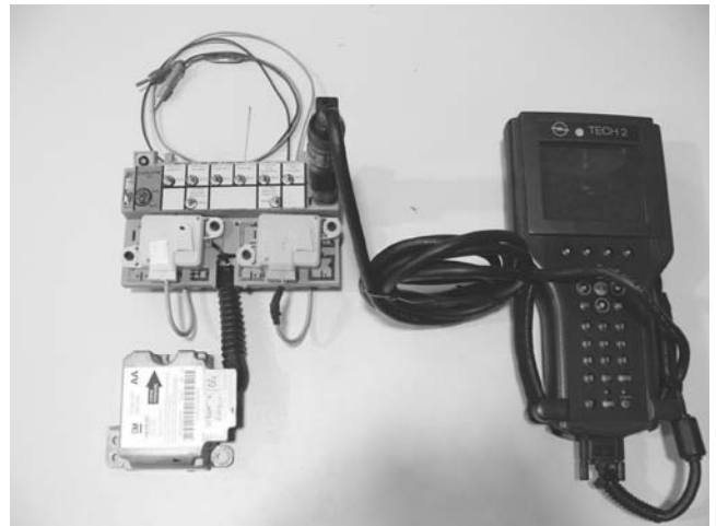
Fig. 3. Photo of tester of air pillow unit connected with the diagnostic equipment tech2 for Astra Classic model
