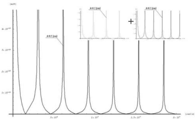
Fig. 21. Characteristics of piezoelectric stack containing two plates with different thickness and in domain of the frequency
