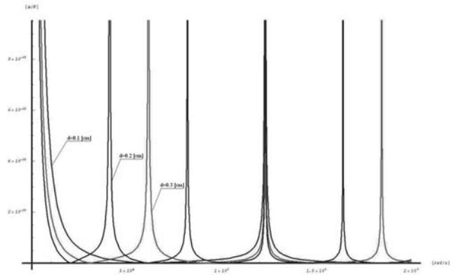
Fig. 16. Characteristics of a single piezoelectric plate in domain of the frequency depending on the thickness of the plate
