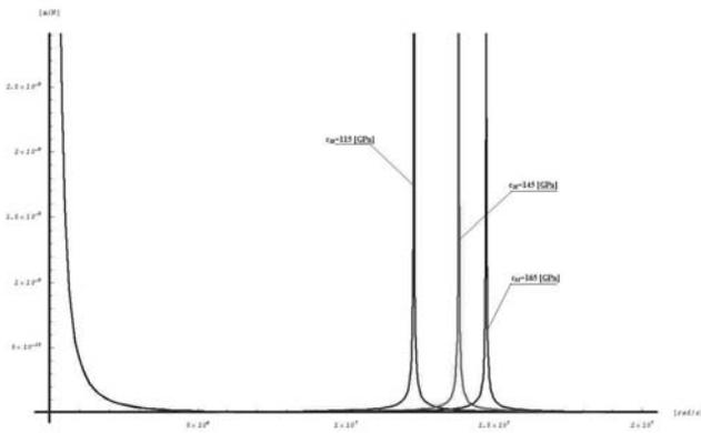
Fig. 19. Characteristics of a single piezoelectric plate in domain of the frequency depending on the module of piezoelectric elasticity
