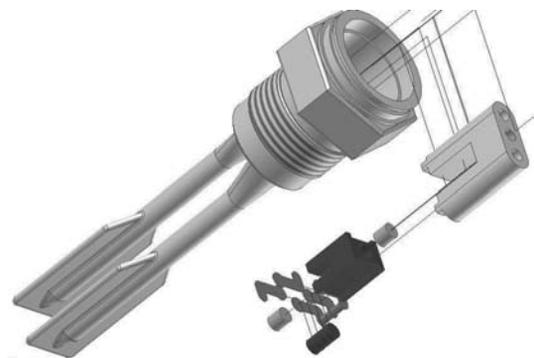
Fig. 23. Construction of level switch
