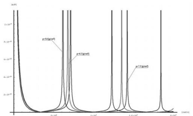
Fig. 18. Characteristics of a single piezoelectric plate in domain of the frequency depending on the piezoelectric density
