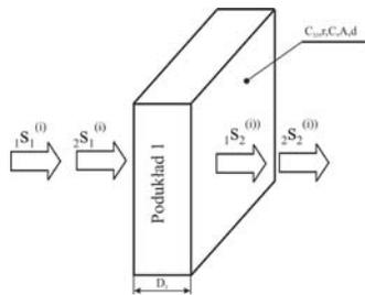
Fig. 14. Model of single piezoelectric plate after reduction
