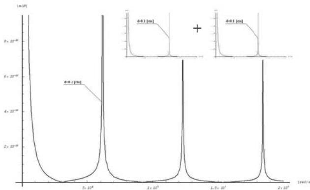
Fig. 20. Characteristics of piezoelectric stack containing two plates with the same thickness and in domain of the frequency
