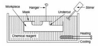
Fig. 1. Typical chemical machining set-up [6]
