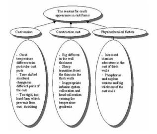
Fig. 3. Examples of the causes of cold crack formation
