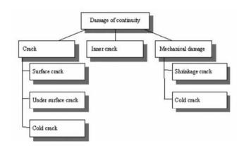
Fig. 2. Example of the hierarchy in casting discontinuities defect
