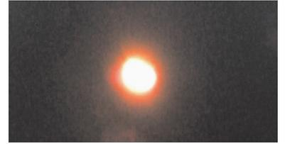
Fig. 7 Output beam spot of WBC after coupling mirror with injection current of 60.6 A
