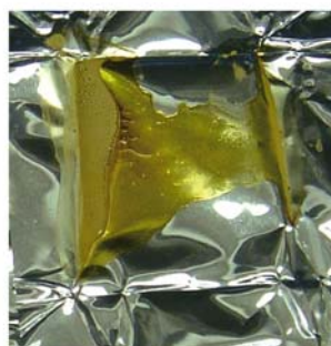
Fig. 3 Photo of 6% PMDA/4,4'-ODA film after 300 °C under Ar atmosphere
