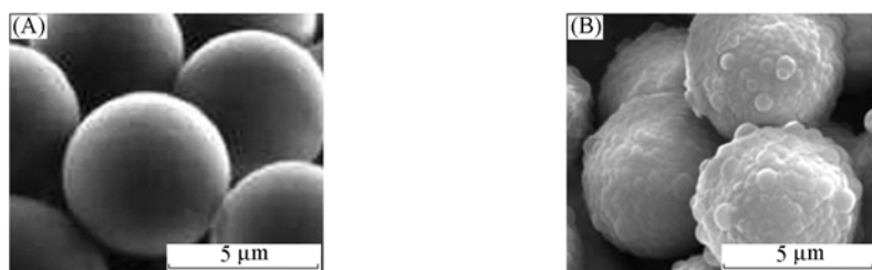
Fig. 1 SEM images of bare zirconia sphere (A) and polystyrene-encapsulated zirconia (B)
