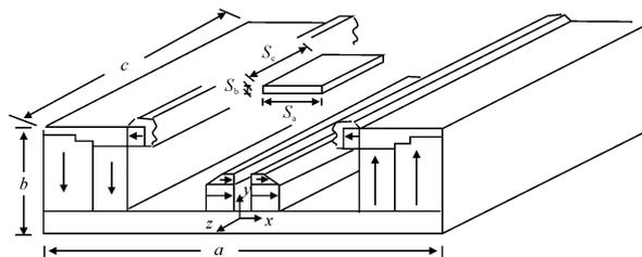
Fig. 10 The 3-D unilateral MRI magnet structure [12] ( $a=80$  cm,  $b=22$  cm,  $c=75$  cm;  $S_a=12$  cm,  $S_b=0.4$  cm,  $S_c=12$  cm)
