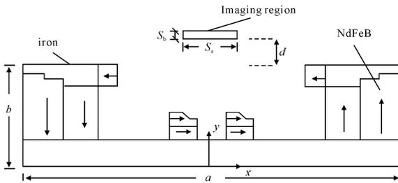
Fig. 8 The unilateral permanent magnet model
