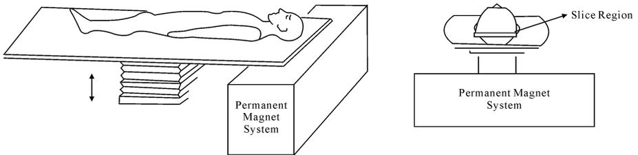
Fig. 1 The unilateral MRI system with a slice imaging region
