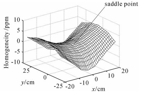
Fig. 3 The distribution of magnetic field in the imaging region
