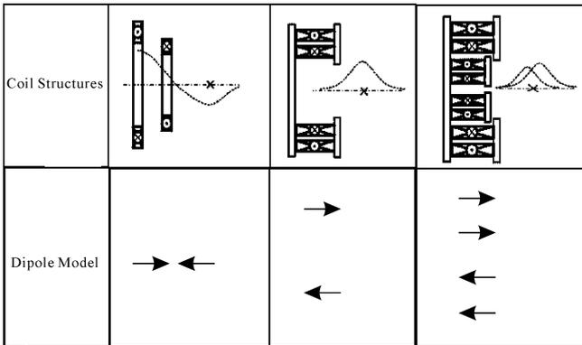
Fig. 5 Unilateral coil structures ("x" represents the saddle point)<sup>[1]</sup>
