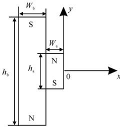
Fig. 6 Opposed permanent magnet blocks
