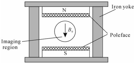
Fig. 2 Four-pole shape MRI magnet model
