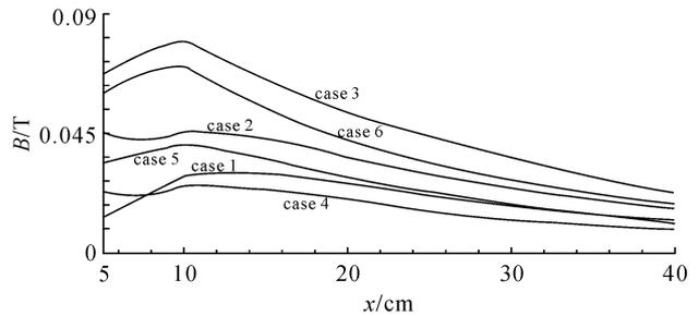
Fig. 7 The value of  $B_y$  at the X-axis for two opposed permanent magnets
