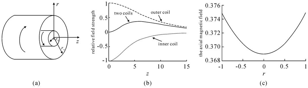
Fig. 4 Opposed coils (a), the magnetic field  $B_z$  at the  $z$  axis (b), the magnetic field  $B_z$  at  $z=5.73$ ,  $-1 \leq r \leq +1$  (c).
