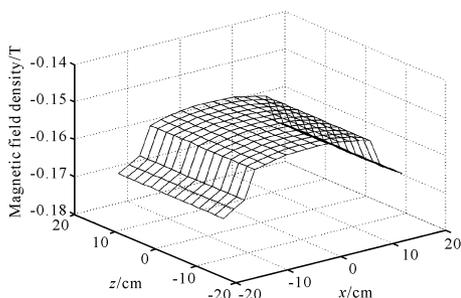
Fig. 11 The magnetic field strength at  $y=24$  cm plane
